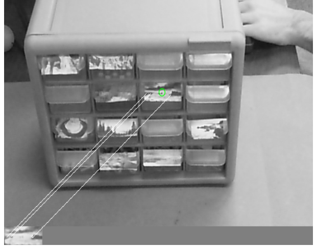
Fig. 5. Image keys were compared with the camera image to find matching features using the SIFT algorithm.
